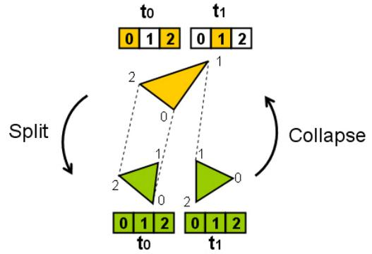
Figure 4. Simplification operation.
