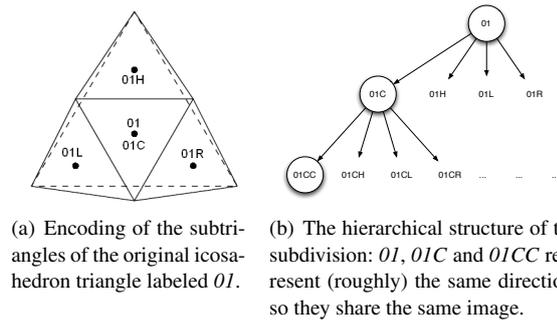
**Figure 1:** Hierarchical structure, encoding and storage of the light field's image data.
