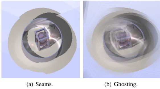
**Figure 3:** Seams and ghosting in a DPP light-field representation of 1280 directional samples.
