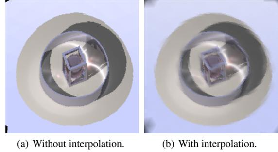
**Figure 2:** Two renderings of a light-field model with 20480 directional samples. The model was obtained by ray tracing a geometric model with multiple light sources, reflection, refraction, and caustics. The spatial resolution of each light-field image is  $256 \times 256$  pixels. The rendering resolution is  $512 \times 512$  pixels.
