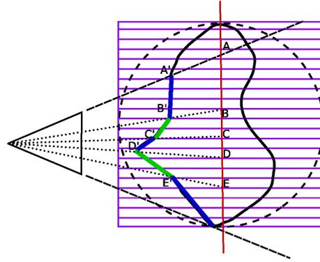
**Figure 4:** 2D analogy of the depth-map approximation to an object's surface. At rendering time rays are cast starting from the eye and passing through the triangles' vertices. Instead of intersecting the rays with the support plane of our original representation (points A, B, C, ...), we use a depth map to get a better approximation to the object's surface (points A', B', C', ...).
