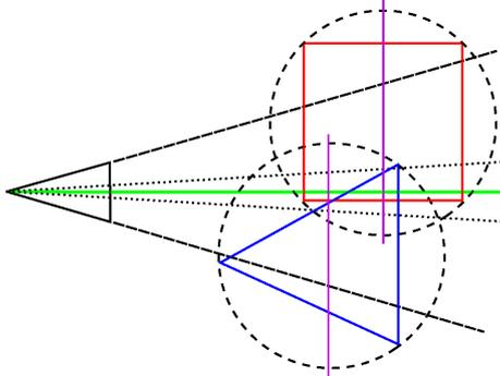
**Figure 6:** The red square is in front of the blue object along the green direction. However, its proxy (in pink) is not, and the blue object appears in front of the red square in a multi-light-field rendering without depth information.
